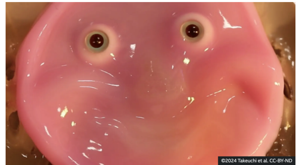
Taking inspiration from human skin ligaments, the prototype face can be made to smile
